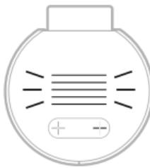
All LED strips will flash three times and the + / - buttons will flash steadily, the device will go into PAIRING MODE for 5 minutes.
