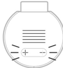
*All LED strips will flash 3 times and the + / - buttons will start flashing steadily, the device will go into PAIRING MODE for 5 minutes.).*
